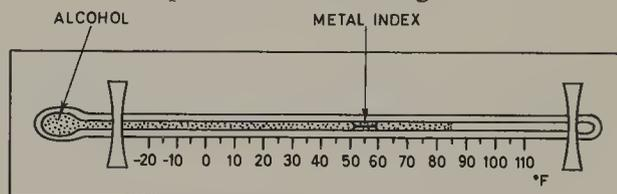
When the temperature rises the alcohol expands. The index does not move but remains in the position to which it was pulled. The minimum temperature is obtained by reading the scale at the end of the index which is nearer the meniscus. In the diagram this is 60°F. By raising the bulb of the thermometer the index is returned to the meniscus.
