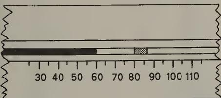
When the temperature falls the mercury contracts and the index remains behind. The maximum temperature is obtained by reading the scale at the end of the index which was in contact with the mercury. In the diagram this is 80°F. The index is then drawn back to the mercury by a magnet.
