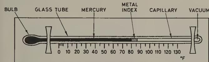
When the temperature rises the mercury expands and pushes the index along the tube.
