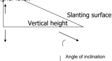
• The vertical height of the inclined plane is the distance moved by load while the slanting surface is the distance moved by the effort.
