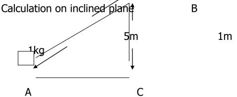
Calculate the work done if the load is moved from A to B.
