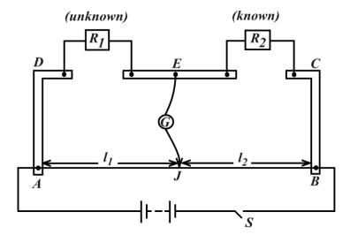
A meter bridge works on the same principle as the wheatstone bridge.
