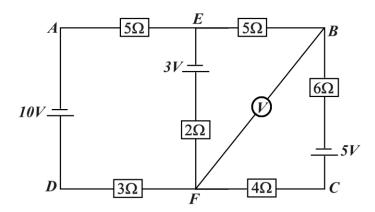
If a very high resistance voltmeter is connected across BF, what will be its reading
