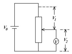
Consider two resistors  $R_1$  and  $R_2$  connected in series to a DC supply of voltage,  $V_0$  and negligible internal resistance as shown in the diagram above for a fixed potential divider.
