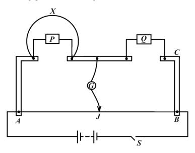
A resistance wire x of cross -sectional area 1mm<sup>2</sup> is connected across P so that the balance point is 66.7cm from A. If the resistivity of X is  $1x10^{-5}\Omega m$  and the resistance wire AB of the meter bridge is 100cm, calculate the length of wire X.
