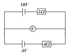
Determine the voltmeter reading.
