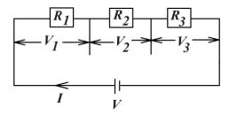
In series arrangement, the current flowing through the resistors is the same but the p.d across each resistor is different.
