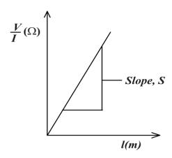
The slope, S is calculated and the resistivity determined from;  $\rho = SA = S \times \frac{\pi d^2}{4}$
