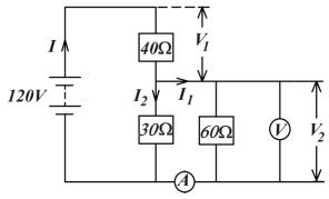
(i) Find the ammeter and voltmeter reading.
