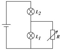
When two identical bulbs are connected in series to a battery of negligible internal resistance, they light normally. The variable resistor R is now connected across bulb  $L_2$ . Explain what happens to the brightness of the bulb.
