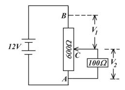
$$R_{AC} = \frac{1}{2}R_{AB} = \frac{1}{2} \times 600 = 300\Omega$$
