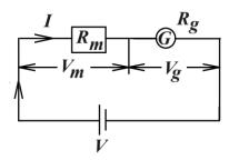
Total P.d to be measured,  $V = V_m + V_g$
