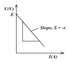
The intercept on the *V- axis* is obtained and is the *emf* of the cell.
