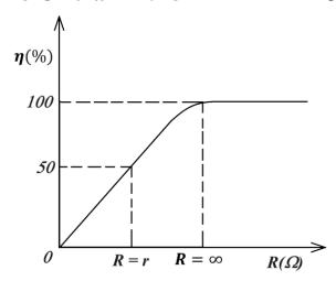
As the load resistance, R increases, the efficiency of the circuit or source increases i.e the efficiency tends to 100% as the load becomes very large.
