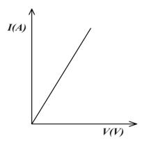
The slope, S of the graph is calculated and the resistance, R is calculated from  $R = \frac{1}{S}$
