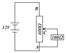
If a load of  $100\Omega$  is connected across the terminals of A and C when the slider is halfway up the divider, find the
