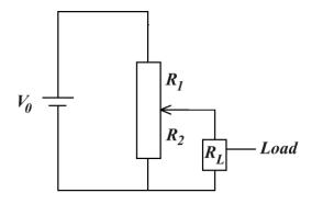
$R_2$  and  $R_L$  are in parallel and so the effective resistance is given by;
