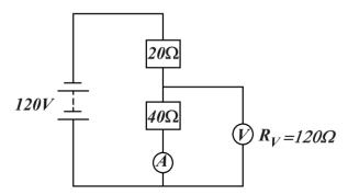
For parallel arrangement,  $R_P = \frac{40 \times 120}{40 + 120} = 30\Omega$
