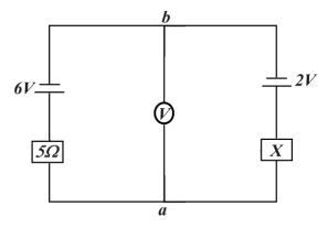
If the voltmeter reads 3V, find the value of resistance x.
