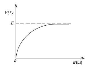
As R becomes very large, less current flows from the source and the p.d across the terminals of the source (i.e terminal p.d) tends to the emf, E of the source.
