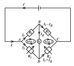
In the circuit above, G is a center zero galvanometer.
