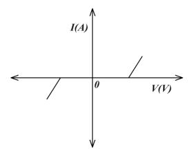
There is no current that flows for very low p.ds until after when the applied p.d is greater than a certain value. This is because the back emf in the electrolyte setup opposes the flow of current through the electrolyte, until the p.d applied is greater than the back emf.
