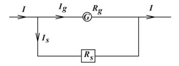
In this case,  $I_g$  is the full scale deflection of the galvanometer.
