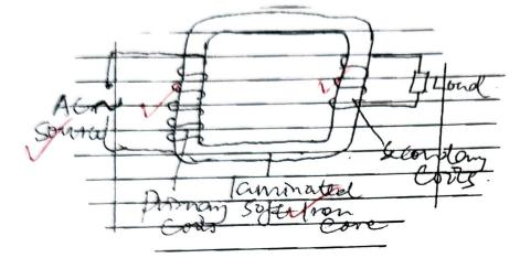
The Ac connected in the primary coil causes a changing magnetic field in the secondary coil.
