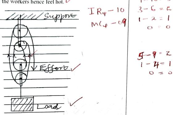
The effort applied to the system through a string is multiplied many times in the pulley system hence lifting the load. I reducing the contact time with the hall of reducing
